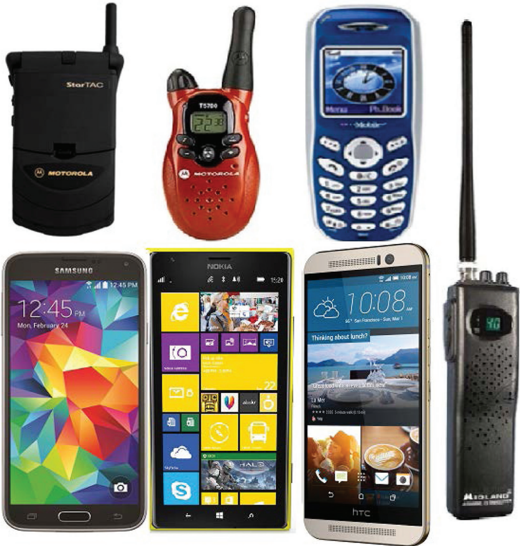
Figure 4.25 Examples of external and embedded/internal antennas used in commercial cellular and CB radios. (SOURCE: Reproduced with permissions from Motorola, Inc. © Motorola, Inc.; Nokia; Samsung © Samsung; Microsoft; HTC; Midland Radio Corporation © Midland Radio Corporation).
